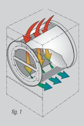
bottom to the top, fall and separate throughout the entire cylinder (see fig.1). Simultaneously, heated air is pushed through and around the load—eliminating hot spots and expediting the drying process.
